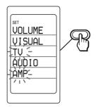
The component names are displayed on the labels. To change the labels, press the SCROLL button. Each time the SCROLL button is pressed, the labels change as in Step 4 on page 14.
